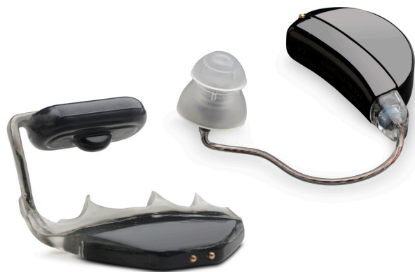
Figure 8 SoundBite™, an in-the-mouth bone-conduction device with implant for tooth attachment and behind-the-ear sound processor. Note: Image provided courtesy of Sonitus Medical.
