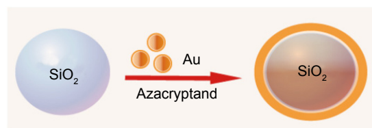
Figure 4 Schematic representation of synthesis of silica–gold nanoparticles.
