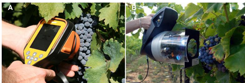
Figure 7 Spectron (A) and Multiplex (B) hand-device sensors for grape quality proximal monitoring, which allows quality maps to be realized.
