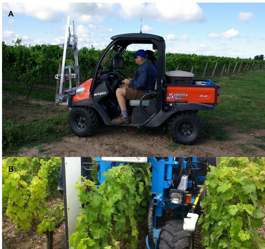
Figure 5 The Trimble ® GreenSeeker ® multispectral sensor for canopy monitoring, carried on a quad (Practical Precision Inc., Tavistock, Canada) (A) or tractor (Avidorhightech SA, Le Mont-Pélerin, Switzerland) (B).
