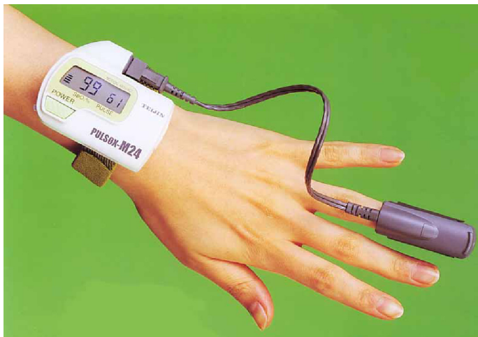
Figure S1 We developed the watch-type pulse oximeter (PULSOX-M24, TEIJIN) in collaboration with Minolta Co. Ltd. The probe is attached to the ring finger, because of ease of pinching.
