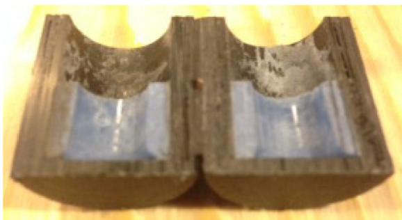
Figure 5 Measurement of the cement height by cutting cement holding cup into half using the band saw machine.
