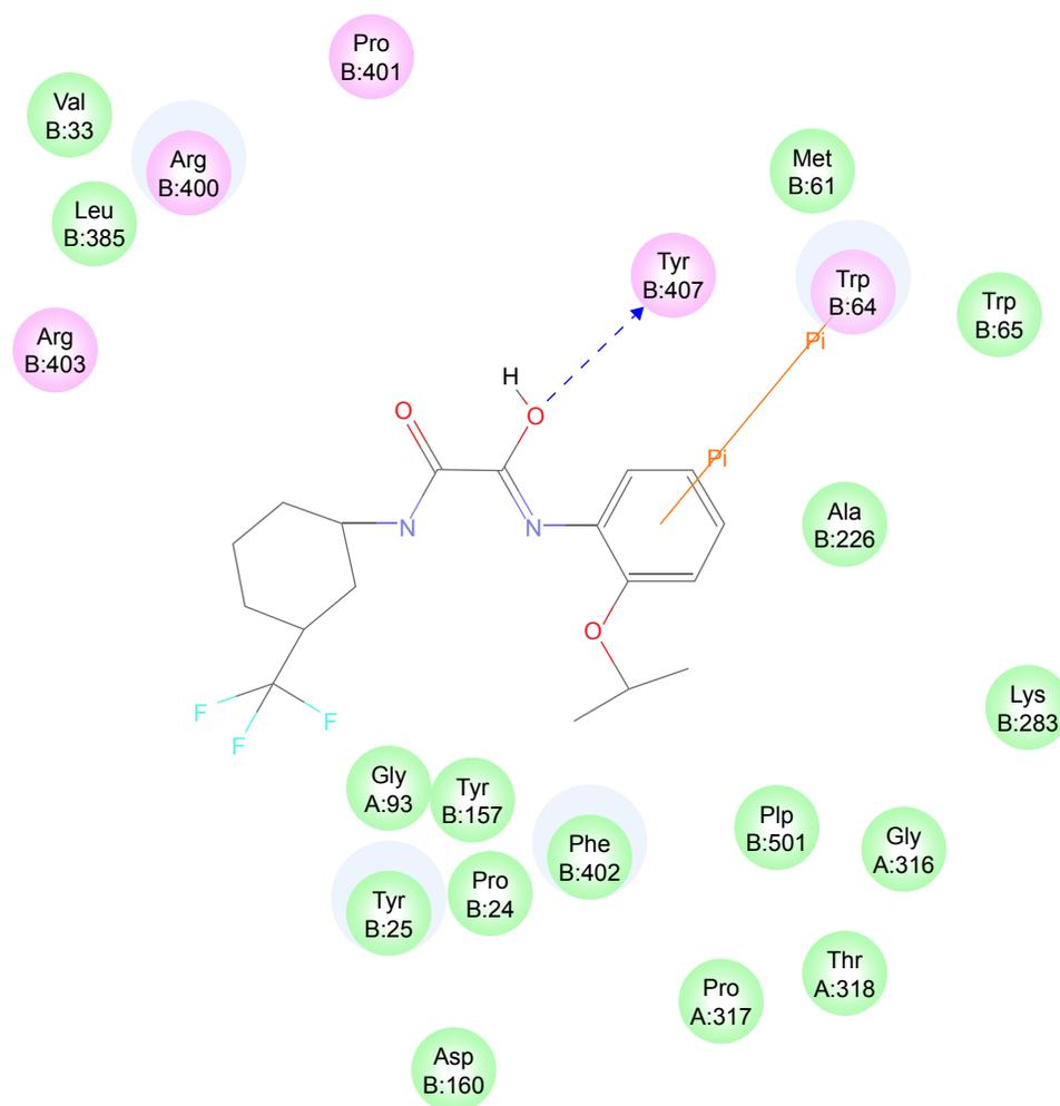
**Figure 5** Interaction diagram for BioA–compound **7** complex. Interaction diagram legends include: 1) pink circles = residues involved in hydrogen bond, charge, or polar interactions; 2) green circles = residues involved in van der Waals interactions; 3) blue circles = water molecules; 4) blue dashed arrow directed toward the electron donor = hydrogen bonding with amino acid side chains; and 5) orange line with symbols = pi interactions.
