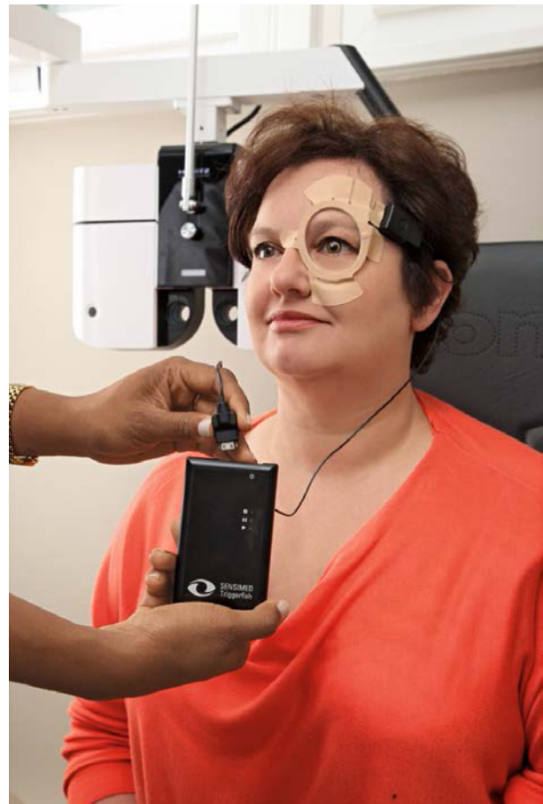
Figure 2 External photograph of the Triggerfish contact lens sensor orbital antenna. Note: Used with permission from Sensimed AG, Lausanne, Switzerland.
