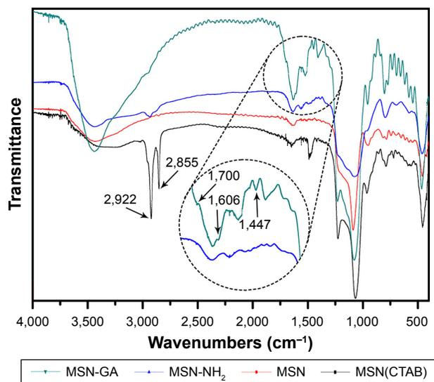
**Figure 2** FTIR spectra of MSN(CTAB), MSN, MSN-NH<sub>2</sub>, and MSN-GA.
