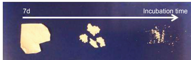
Figure S3 Pictures of the hybrid fibers after several weeks of incubation in SBF.
