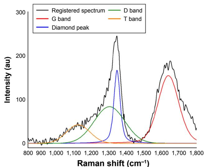
**Figure S2** Raman spectra of diamond nanoparticles.
