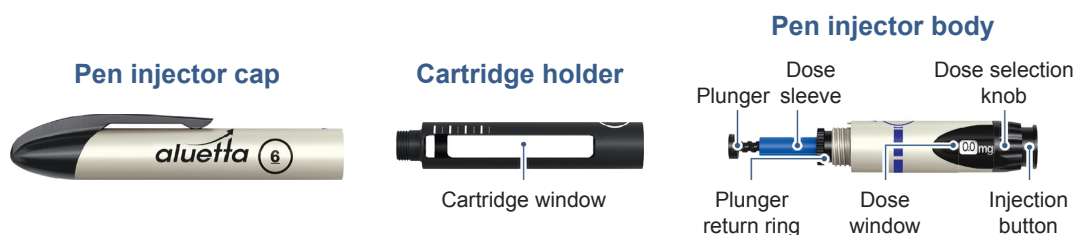
Figure 1 Components of pen device.
