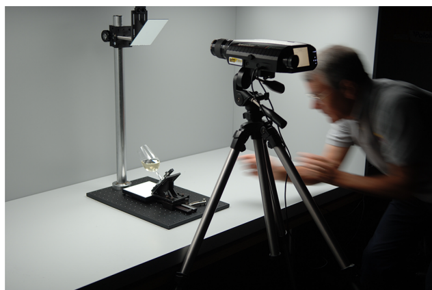
Figure 1 Experimental setup for measurement of wine transmittance in situ within a D65 standard viewing booth.
