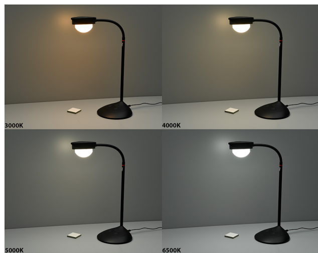
Figure 36 Images of the Fiilex V70 desk viewing lamp in the D65 viewing booth.
