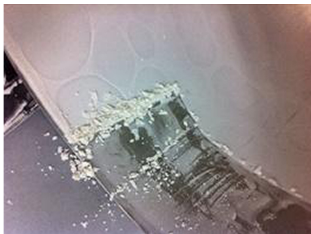
Figure 1 Photograph showing particles stuck to the spray-drying chamber.
