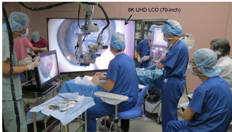
Figure 2 8K UHD microscopic camera for ophthalmic surgery in the operating room site. Abbreviation: UHD, ultra-high-definition.
