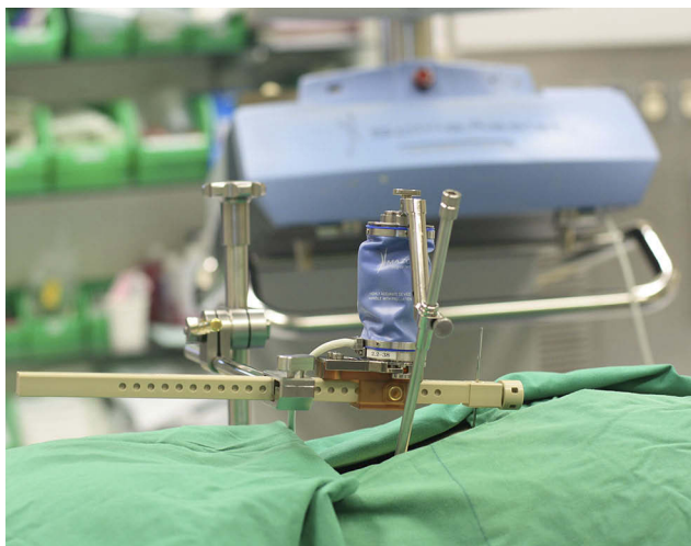
Figure 1 Following the pre-operative CT, the SpineAssist robotic platform is attached to the spine for final image registration.
