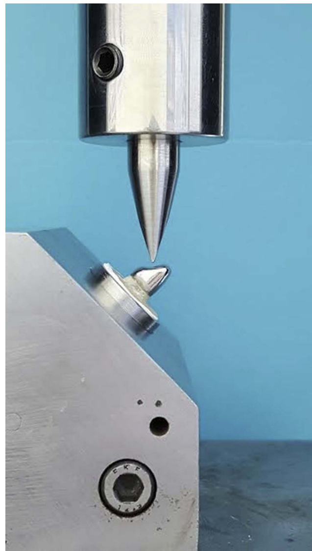
Figure 3 The image shows custom-made assemblies, starting from the superior part; the chisel head is pointed at 135° on the palatal surface of the tested tooth.
