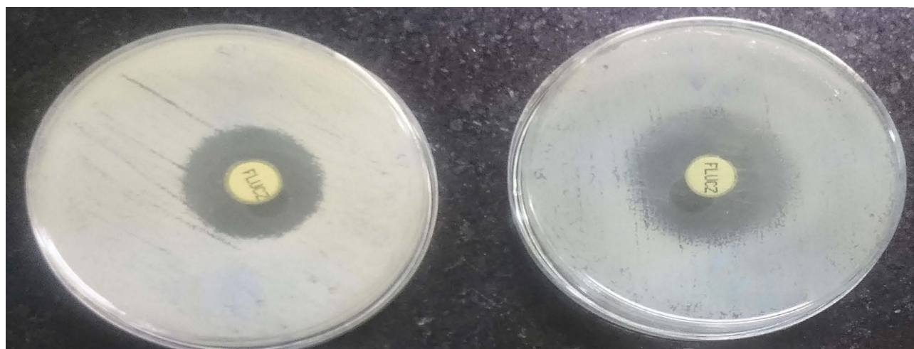
Figure 2 Susceptibility pattern of C. albicans isolates to Fluconazole (25 µg) showing different sizes of inhibition zone: (A) 14 mm (R), and (B) 22mm (S).
