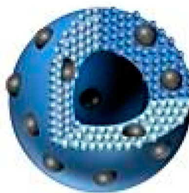
Figure 3 A schematic illustration of silver-loaded titanium dioxide nanocapsule.
