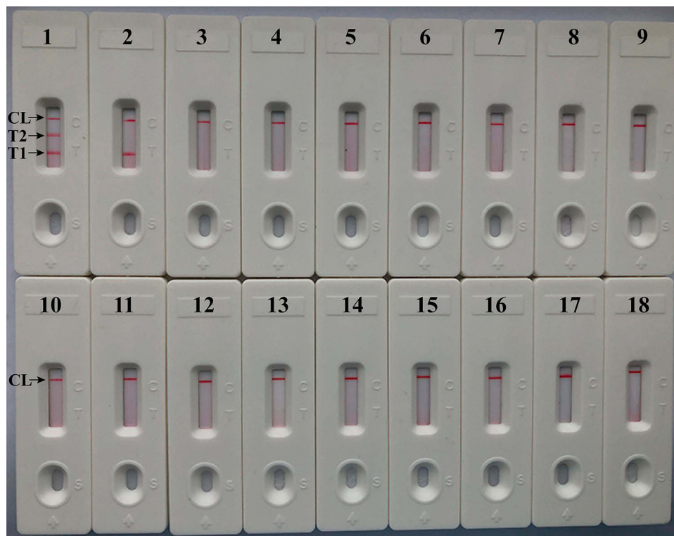
Figure 7 Analytical sensitivity of m-LAMP assay using different bacterial strains. The m-LAMP amplifications were performed using different genomic DNA templates and were monitored by means of visual format. Biosensor 1, MRSA (ATCC 43300); biosensor 2, MSSA (ATCC 25923); biosensor 3–17, biosensor 18, negative control (DW).
