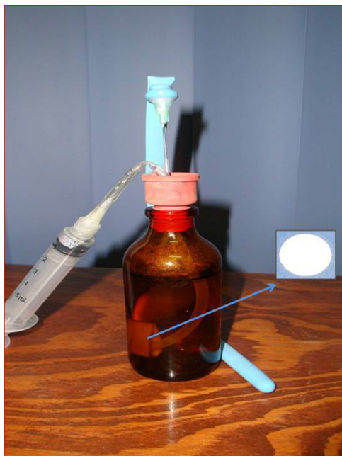
Figure 1 Set-up for the study of dopamine release from silica reservoirs. The experiments were performed in amber glass bottles and under nitrogen atmosphere in order to prevent dopamine oxidation.
