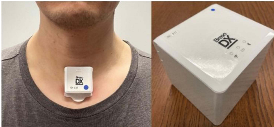
Figure 1 The BresDX1 and its computing module, which simultaneously collects trachea-sternal motion and tracheal sound from the BresDX1 and SaO 2 from the pulse oximeter.
